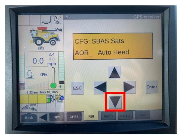
Once the "E" on AORE is flashing, push the down arrow until 138 appears.
