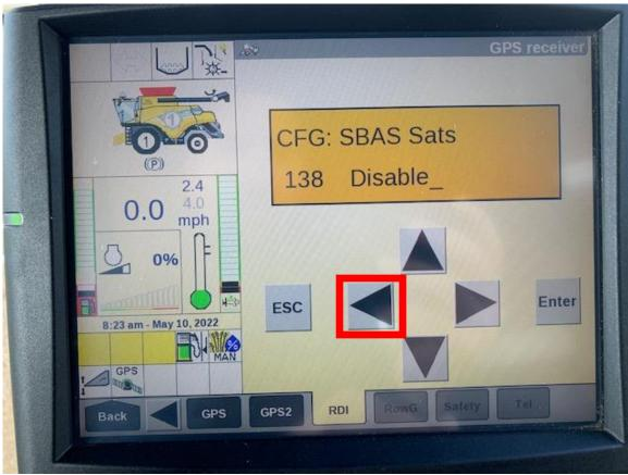
Once 138 shows disabled push the left arrow so the "8" on 138 is flashing
